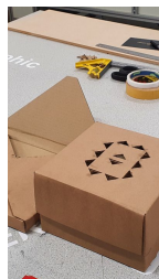
Box prototypes cut from the lazer cutter (03/03/2022)
