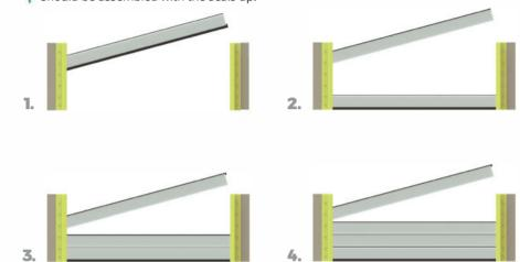
Once all the beams are assembled, place the compression keys in the fixing holes located in the guiding elements and compress the system by turning the handles of the vertical compression screws.
