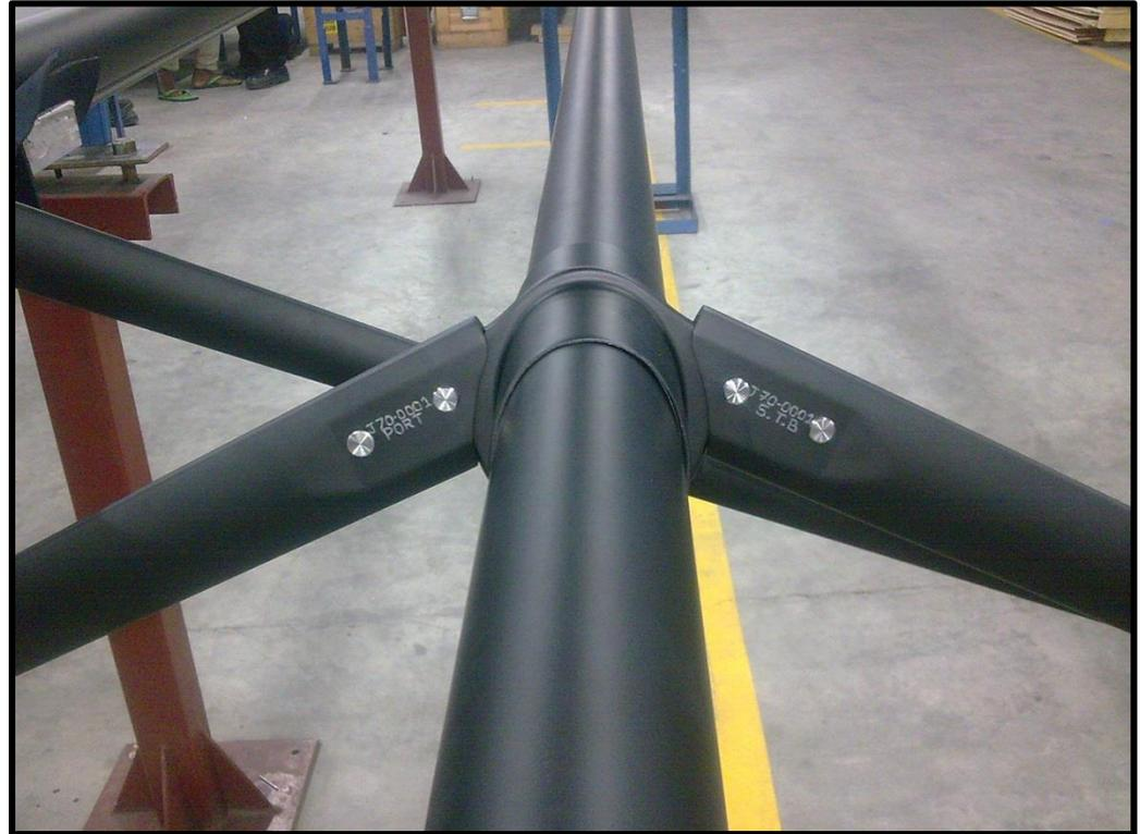
**Hint:** It can be a good idea to tape over the spreader clevis pins & spreader ends to prevent accidental tearing of your spinnaker on hoists & douses. Rubber splicing tape works nicely.
