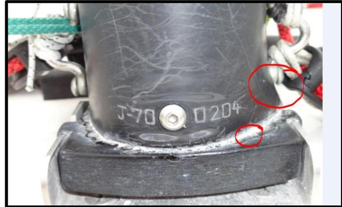
It is recommended that the mast is washed down with fresh water after every sail - making a deliberate point of hosing water through the lower halyard exit slot will flush out any saltwater residue.
