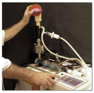
A typical application is the NGI with an anatomical throat and mixing inlet.
