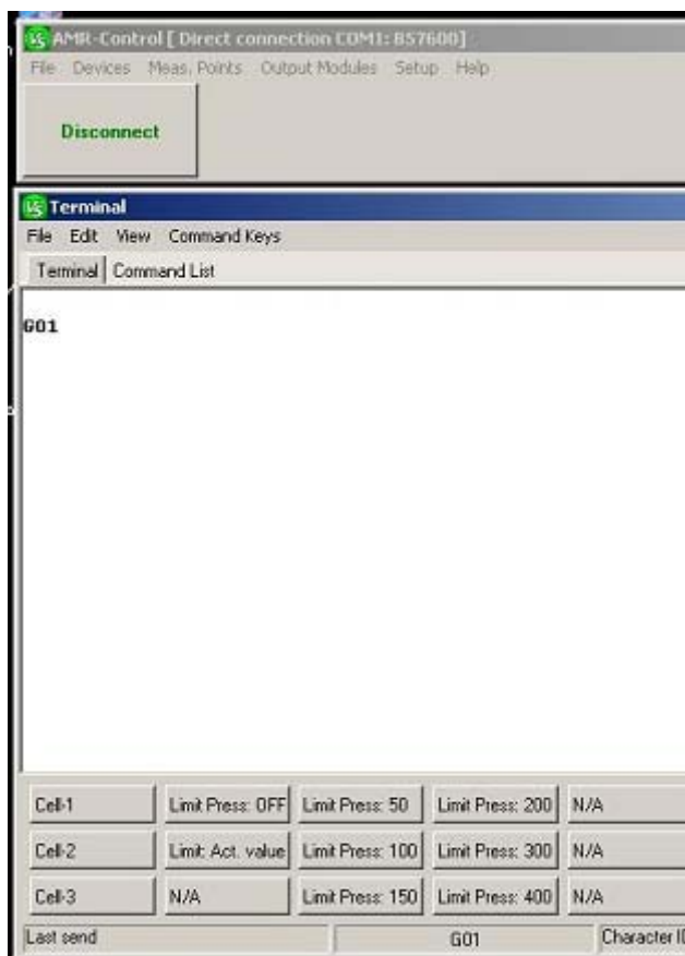
Picture 7. If you would like to change the Max limit of the pressure it is possible to do that by clicking on the Cell no concerned (example: Cell-1 down to the left on the screen).
