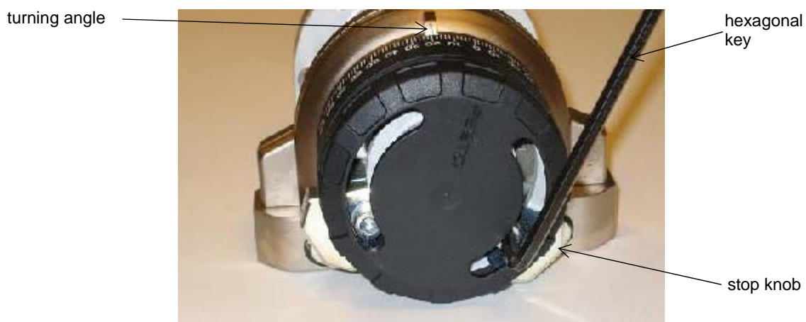
FIG 6. CHEWING APPARATUS: Setting the angle of rotation.
