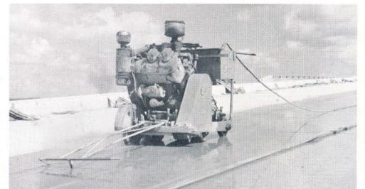
60.5-hp V-461D on concrete saw
