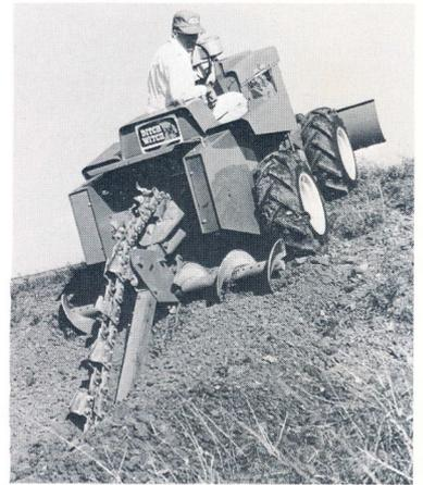
60.5-hp V-461D on trencher-blade
