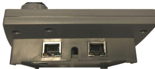
*L-Net ports on the back side of 4E-FMTC*
