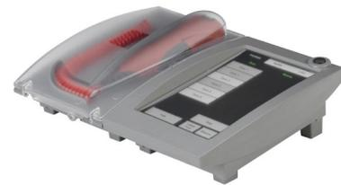
4E-FMT only offers emergency mode operation. While the transparent fireman's microphone door is closed, the panel is locked (access level 1) and no paging functions are available. As soon as the transparent door is open, 4E-FMT automatically switches to emergency mode, where full emergency functionality is enabled. This includes one EVAC message, two ALERT messages, silence/reset functions and a fireman's microphone for live evacuation broadcast, and more.
