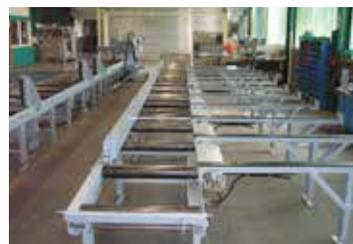
Further length of manual and driven stock roller tracks, on request
