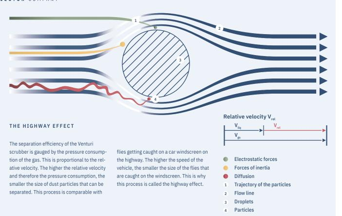
The highway effect reflects the principle of the Venturi scrubber's separation capability.
