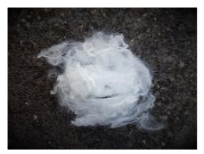
VTT's new study on improvement of Biocelsol process for production of regenerated cellulosic fibres. The limited scalability of cellulose activation and dissolution stages had thus far hindered the commercialization of the Biocelsol technology. The recent development enables continuous production of regenerated cellulosic fibers.
