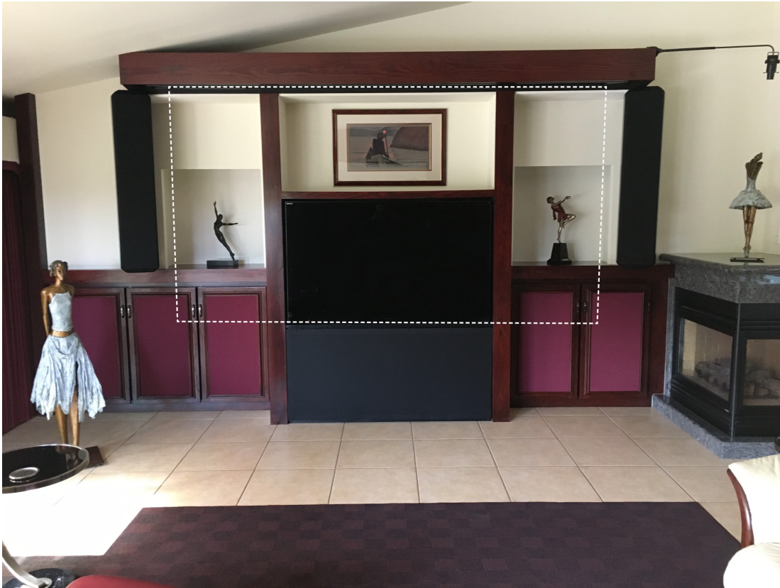
Figure 1. The author’s entertainment/family room showing the dashed outline of the 10 ft motorized front-projection screen. The Revel Salon2s are inverted, tweeters at the bottom placing the soundstage at the right elevation. A Revel Voice2 is under the 65-inch flat-screen monitor with the tweeter as high as possible. The surround loudspeakers are Revel Gem2s, themselves excellent stand-alone loudspeakers. Four JBL HTPS-400 subwoofers in a Sound Field Managed arrangement provide bass (see Section 8.2.8, p. 244). See also Figure 7.21, p. 192.
