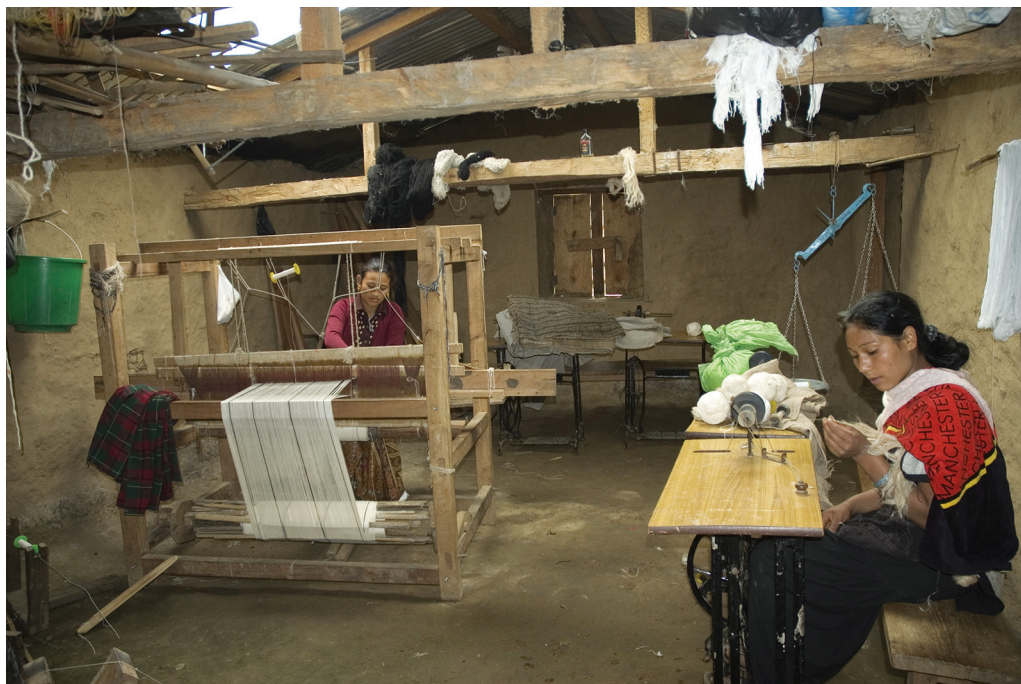
Fig. 27.5: Development projects in Nepal have introduced four shaft-treadle looms and spinning wheel used in more settled environments in the domestic sphere. Here, the fibre is spun by hand into a thread much faster than by the use of the traditional drop spindle. However, the drop spindle/hand spindle enables the person to spin while walking, shepherding or doing other tasks. Before spinning, the fibre bundle is untied by hand and the bundle is kept in order by twisting it around the foot and one toe (Photo: © Ellen Bangsbo).
