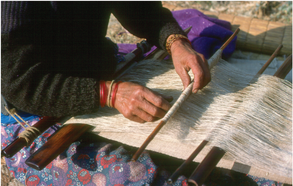
Fig. 27.4: In Nepal, the hand-spun Allo nettle yarn was traditionally woven on backstrap looms, an easily portable loom consisting simply of a warp secured to a beam and kept straight by the strap around the weaver's body. Backstrap looms were used to produce shawls, mats, sacks, headbands, and clothing by local ethnic groups such as Rai, Sherpa, Magar, and Gurung. This photo shows a woman weaving nettle cloth on a backstrap loom in Ghandrung, Nepal 1979 (Photo: © Ellen Bangsbo).
