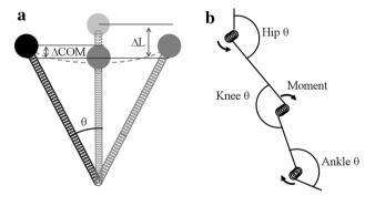
Fig. 1 Biomechanical stiffness models for changes in (a) vertical and leg stiffness [19], and (b) joint stiffness [18] during running. Vertical stiffness is calculated from maximum vertical force and centre of mass (COM) displacement. Leg stiffness is calculated from maximum vertical force and 'leg spring' compression (L). Joint stiffness is calculated from changes in joint angles and moments
