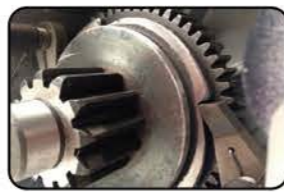
Double-lock brake system
