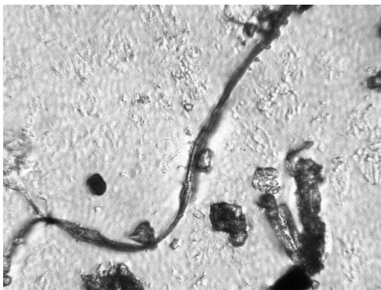
Figure 8. Photograph of contamination from a used firefighter SCBA facepiece, at 400X magnification
