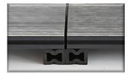
to surface. If the rail is placed next to each other between the ends, a gap of 5 mm must be left. The same gap must be left between the end of the rails and a stationary object (such as a home wall).
