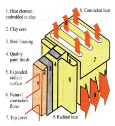
Various test have been completed on these radiators in Germany over the years These have demonstrated the benefits of the retained heat
