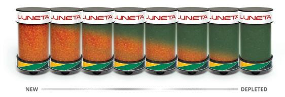
The D-Series is constructed of industrial grade raw materials, tested to ensure a wide range of chemical compatibilities, and features high impact resistant ABS top and bottom caps. The clear acrylic tube makes it easy to inspect the condition of the color-changing silica gel from a distance. The silica gel turns from gold to dark green to visually indicate the adsorption of moisture and confirm the breather is getting the job done.
