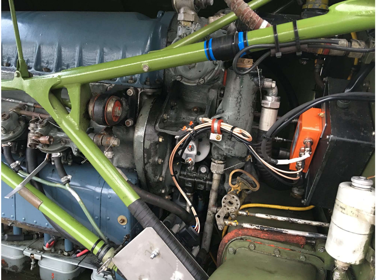
CVI-4 Installation on Gipsy Major – DH Chipmunk, OY-ATD
