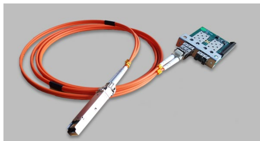
Fig. 1, Mini MADI module installed with bidirectional optical fiber and SFP
