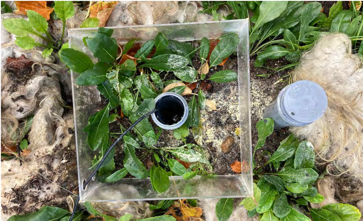
Fig. 100 - 102. Images of the development of the speculative prototype for the second outdoor experiment. The box is 25x25cm and 10cm in height. It is made of transparent plexiglass and has a lead of in a semi-transparent tone for reject the sunlight on the earthworms' skin, but still providing possibilities for counting the earthworms appearing within the frame of investigation. Besides the main frame-box there is made an extra box for the recorder to lay in, avoiding being wet if it rains during a recording. By Permiin, 2022.
