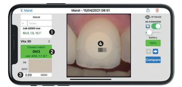
The information on the display of your phone is very clear and shows always the L\*a\*b\* coordinates of the measured tooth in comparison with the values of the closest recognized shade guide in the database.
