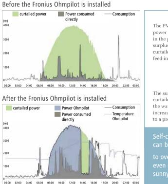
The PV system supplies power to the electrical loads in the property while the surplus energy has to be curtailed due to the zero feed-in limitation.
