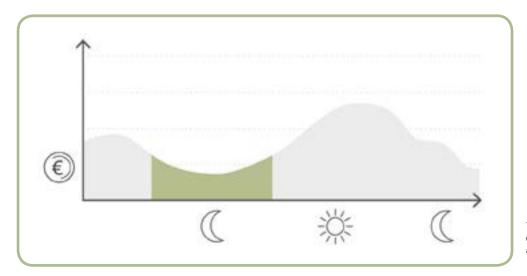
The green area indicates charging an electric car with a variable electricity tariff
