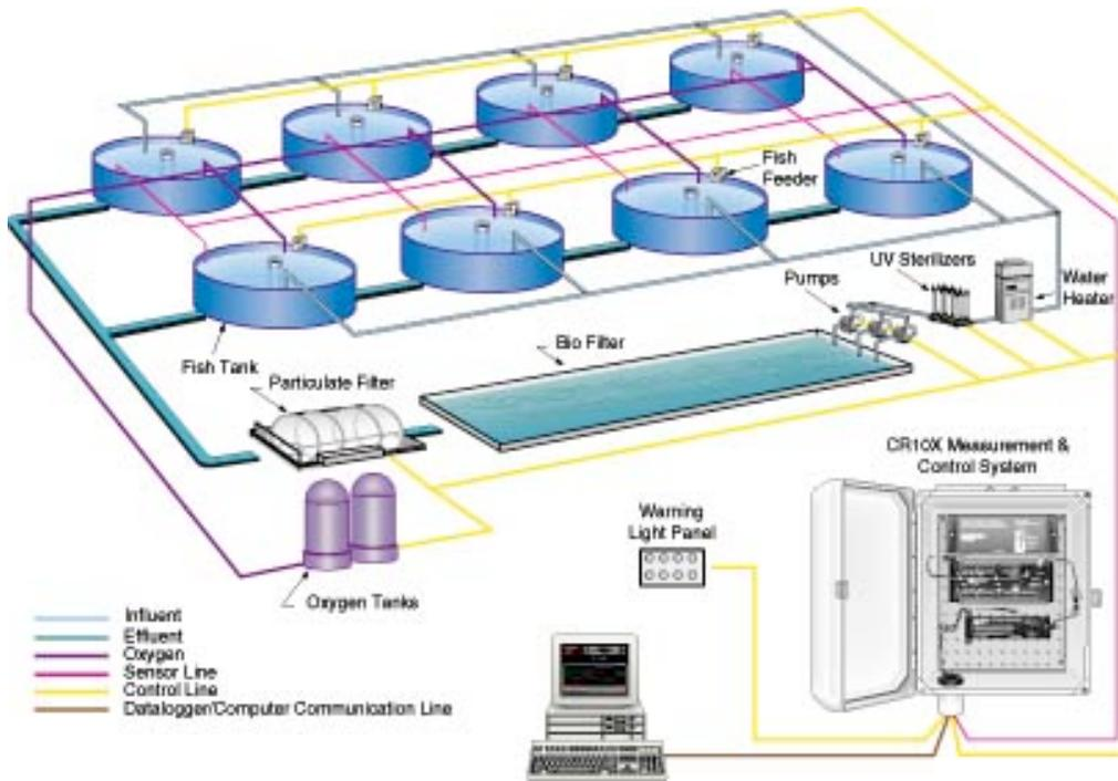
Figure 2: Closed containment system grow-out tanks
