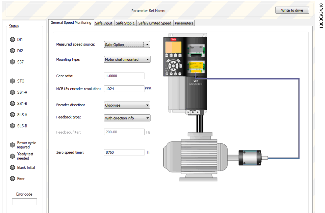
Illustration 19.3 The Opening Tab of the Safe Plug-In for MCB 15x Plug-in Interface (Operating in Offline Mode).
