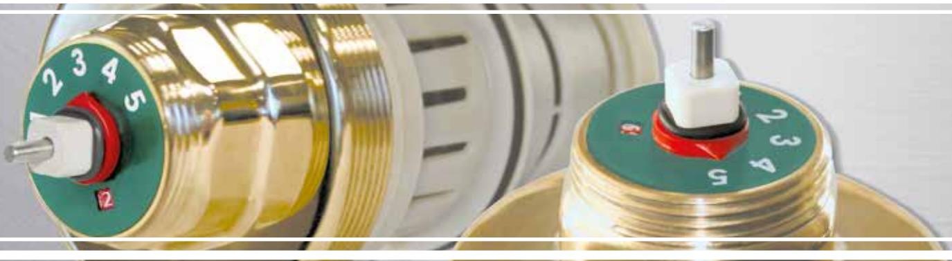
The FlowCon Green inserts ensure that the design flow will never be exceeded and with the matching modulating actuator any flow rate between closed and design flow is obtainable regardless of pressure fluctuations in the system maintaining 100% authority on the actuator always using full valve stroke independent of pre-set maximum flow.
