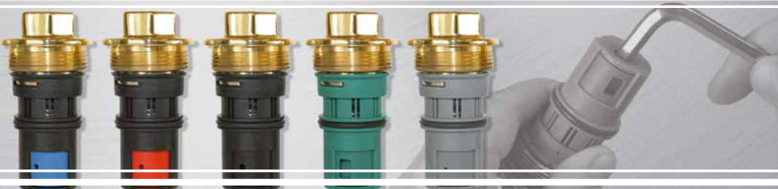
The composite automatic flow rate cartridges ensure that the design flow will not be exceeded regardless of pressure fluctuations in the system.
