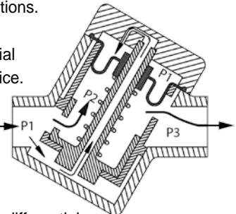
Within the defined pressure differential regulation range the pump supplies sufficient pressure to affect the spring and diaphragm in the cartridge.
