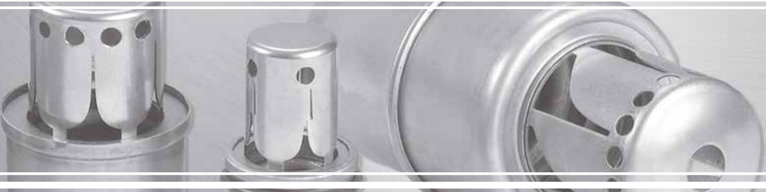
The stainless steel flow rate cartridges ensure that the design flow will not be exceeded regardless of pressure fluctuations in the system. Since the cartridge is factory pre-set, the flow rate cannot be adjusted on the cartridge. The advantage of this type of cartridge is that it works at lower pressure differentials and with higher flows.
