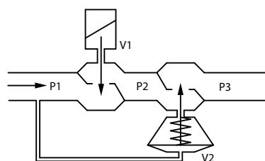
When pre-setting the maximum flow rate, the inlet orifice is changed in size sideways which does not interfere with the length of the stroke. When modulating, the orifice areas are affected by the actuator using the full stroke which results in the fact that the orifice area is changed in size in a vertical movement.
