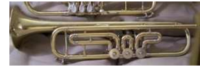
BACH'S EARLY ERROR: VINCENT BACH MADE EARLY ROTARY VALVE TRUMPETS WITH ROTARY VALVES IN THE PISTON VALVE POSITION FURTHER DOWN THE AIR COLUMN. SHOWN HERE IS A 1934 MODEL 7 . THESE WERE NOT SUCCESSFUL AND ONLY 15 WERE MADE. BACH'S LATER AND CURRENT ROTARY VALVE INSTRUMENTS HAVE THEM IN THE CORRECT POSITION.
