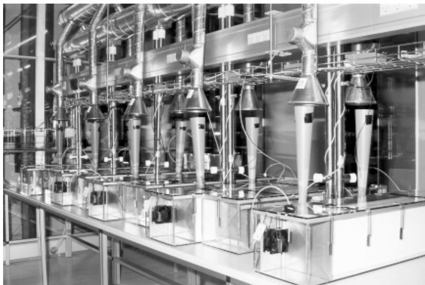
Figure G2. CLIMPAQs supplied with air from an external supply air system.
