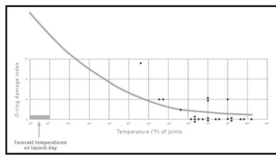
The curved line is a mean derived from the data points—actual on the right half, extrapolated on the left. The higher the line, the greater the anticipated damage to the o-rings.
