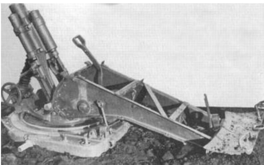
7.85 cm lightweight mine launcher, new style, with maximum barrel elevation.
