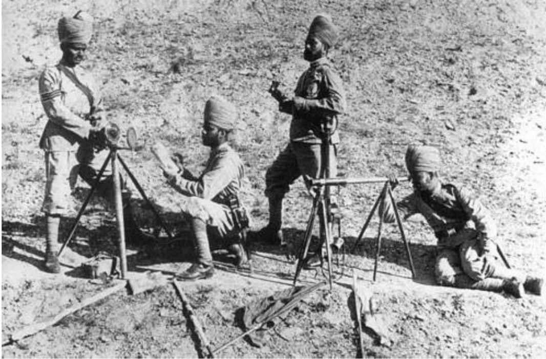
Optical signaling with heliograph by 1st Grenadier Regiment of Bombay Infantry, 1897. From Source 5.
