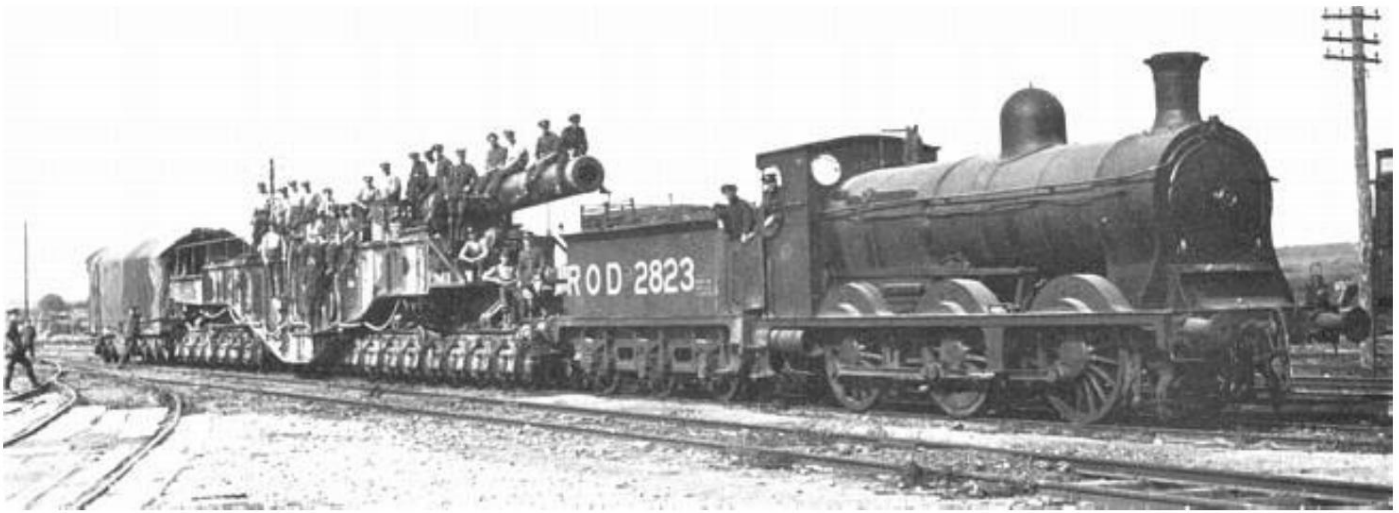
His Majesty's Gun "Boche Buster" (14-inch railway gun) in transport position. From Source 5.
