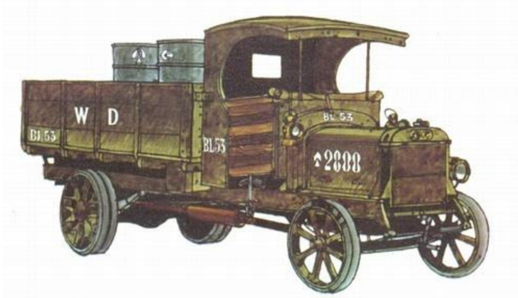
AEC B-type bus converted to truck.
