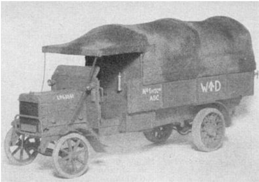
LGOC B-type bus in truck version.
