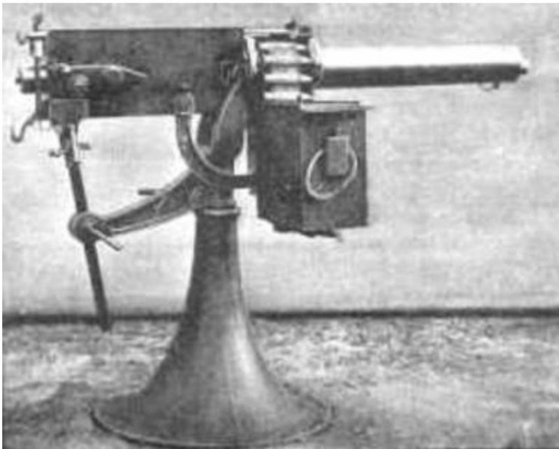
37 mm (Pom-Pom) machine gun, in stationary mount. From Battlefield Anomalies, Second Boer War, Artillery .
