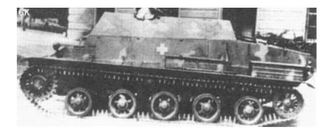
In 1943, a very limited number of vehicles were built/converted to armored personnel carriers with the type designation 43.M Lehel. Basically, it is a Nimrod anti-aircraft tank without a turret, but with low fixed sides.
