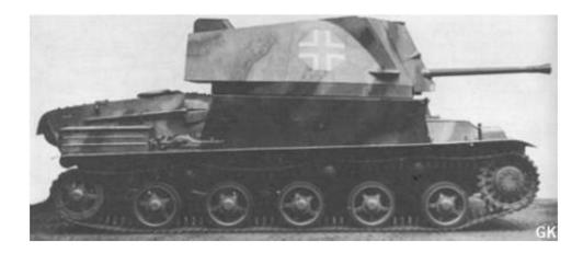
In 1941 Hungary obtained licensing rights to manufacture the Landsverk L62 anti-aircraft tank and a prototype was shown in October 1941. I assume that they had the opportunity to utilize both machinery and experience from the manufacture of Toldi tanks, which were manufactured from the Landsverk L60 type.
