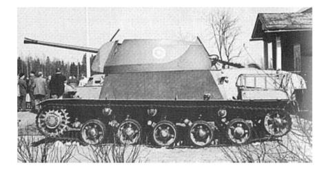
The Landsverk L62, as the type was designated by the factory, basically consisted of a Landsverk L60 chassis, on which was mounted a turret with a 40 mm anti-aircraft gun L/60.
