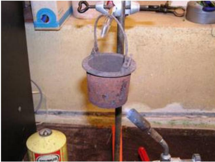
1. Under primitive conditions without temperature control, the tin is heated.
