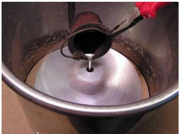
2. & 3. The mold is brought into rotation in the "machine" and the liquid tin is poured into the center hole.
