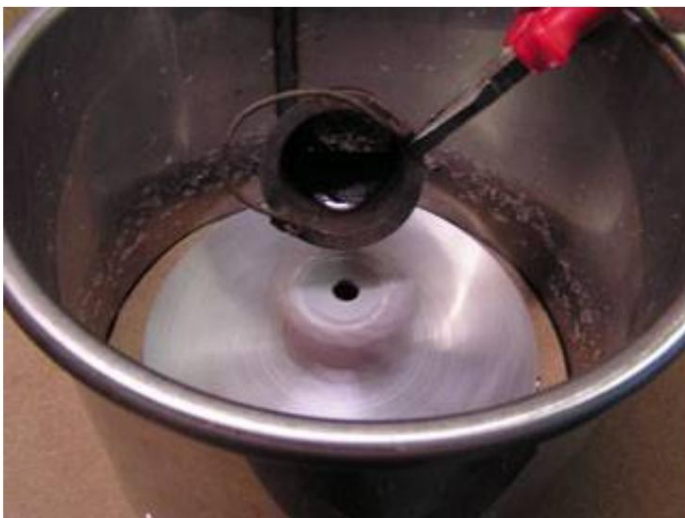
2. & 3. The mold is brought into rotation in the "machine" and the liquid tin is poured into the center hole.
