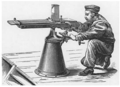
Nordenfelt machine gun, in five-barreled version. Fra Hotchkiss, Gardner and Nordenfelt Guns (An Illustrated Treatise on Ammunition and Ordnance, 1860-1960).
