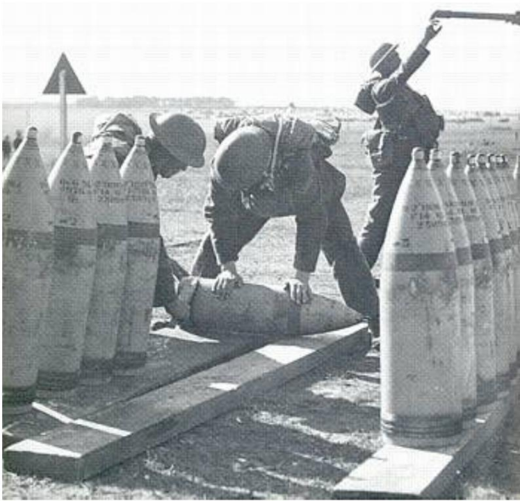
Preparations are being made to load a 9.2" howitzer. The "treadmill" of the grenades is cleaned of dirt with a wire brush. From Source 2.
