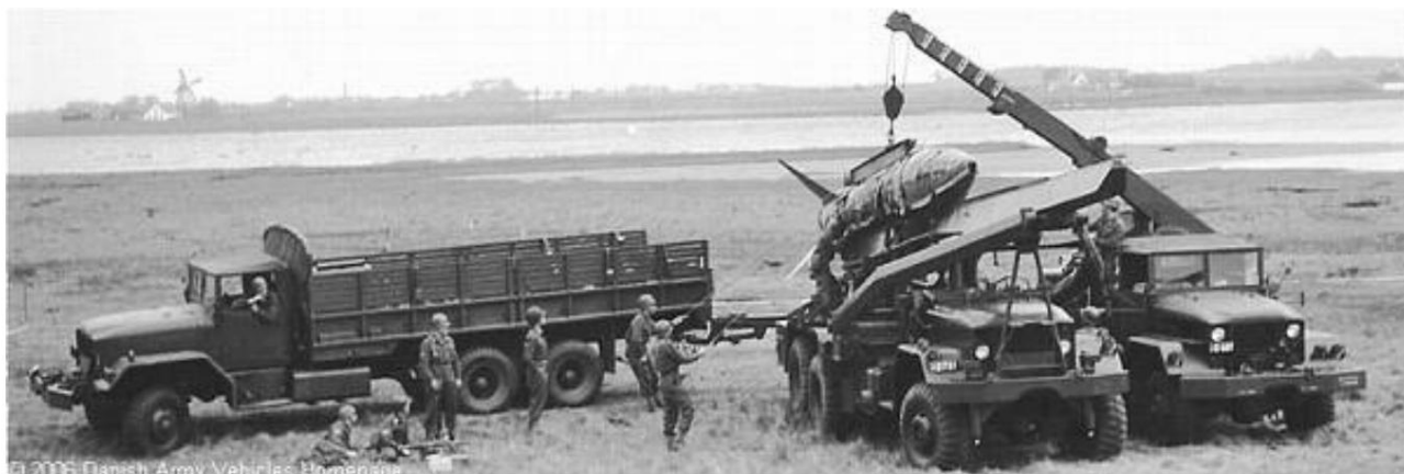
Some of the components of the Honest John rocket system: M55 rocket carriage, M289 rocket guide and M62 crane carriage.
