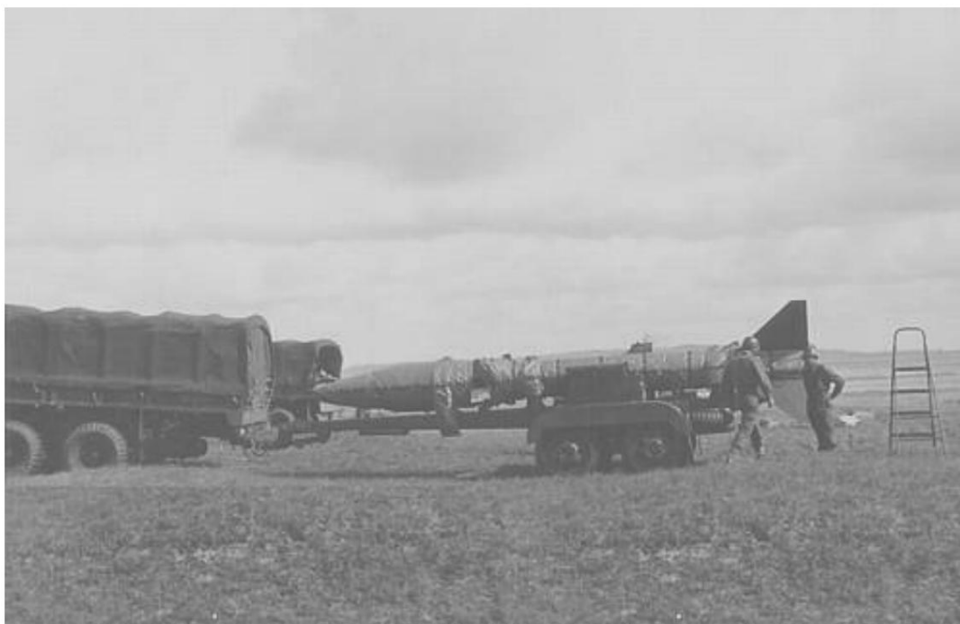
Some of the components of the Honest John rocket system: M55 rocket carriage, M289 rocket guide and M62 crane carriage.
