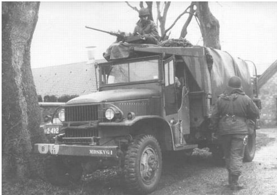
2 1/2 t GMC, 6x6, CCKW-353, truck, with 12.7mm machine gun M/50 in anti-aircraft car mount M/50.
