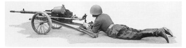
20 mm machine gun, set up to fire from the transport wheels. (Danish Industry Syndicate). From Source 10 6).
