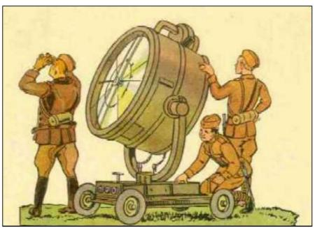
The searchlight is of the type used in the army. Its range is 10-12 kilometers and the brightness corresponds to 800 million normal lights. It was transported on a two-axle truck (Kraftvogn Model 1934, which was a Danish Triangel truck), from where it was rolled down a chute to the operating position on the ground. The searchlight was powered by a dynamo on the truck. The searchlight could be linked together with the anti-aircraft guns so that it could automatically work in sync with the guns.
