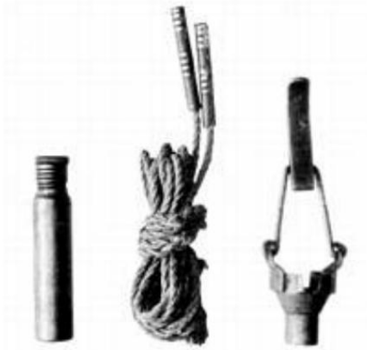
Cleaning props for the 1889 system: Oil bottle, wiper cord and wear cap. Formed after illustration in Source 1.
