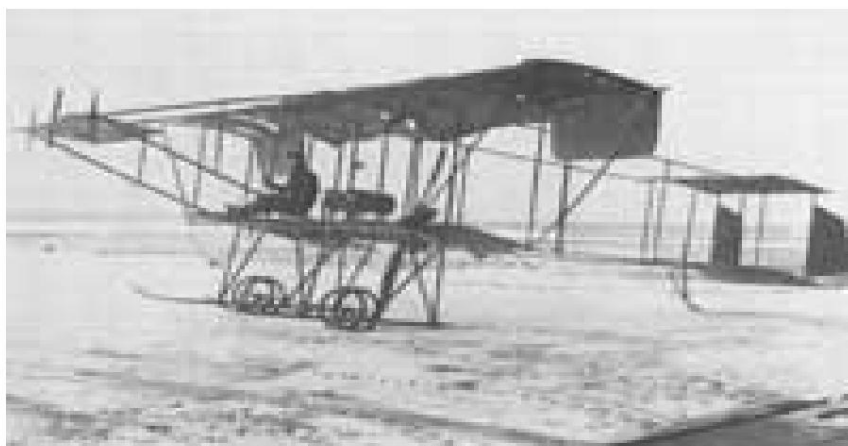
The aircraft Glenten, the navy's first aircraft, had a 50 hp engine and a top speed of 80 km/h. (Photo from Orlogsmuseet archive)
