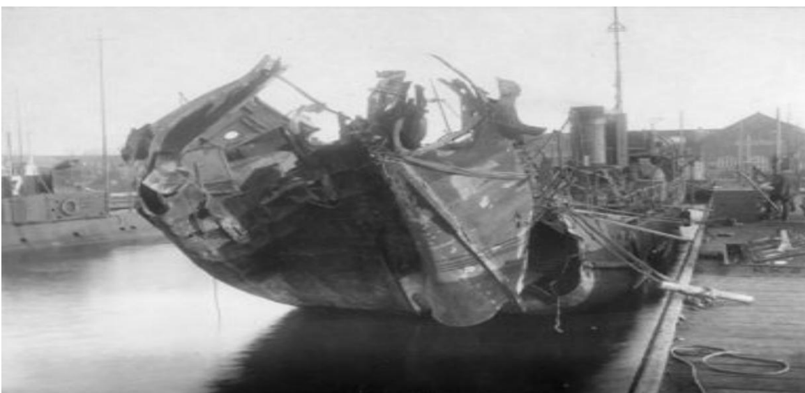
The torpedo boat Sværdfisken is seen here after returning to Holmen with the stern ship blown away, on the left in the picture the submarine Nymfen can be seen. (Photo from Orlogsmuseet archive)
