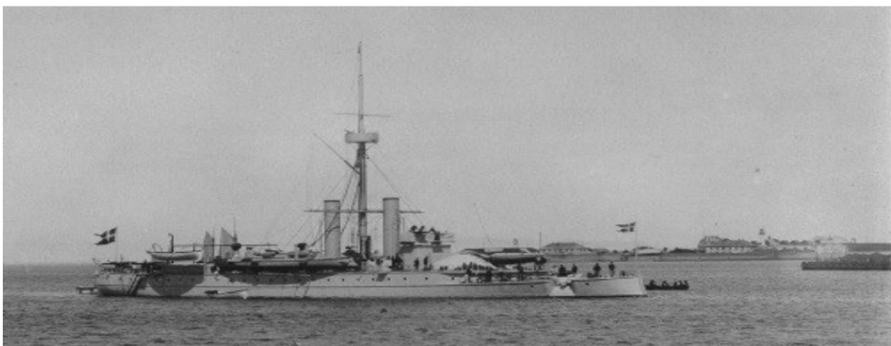
The armored ship Tordenskjold 1884 in color 2 with the two 2nd class torpedo boats on board - No. 4 on the port side and No. 5 on starboard. The difficult rough between the chimneys was used for launching and launching the torpedo boats. (Photo from Orlogsmuseet archive)
