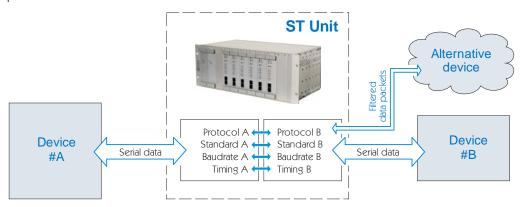
Used as MUX, the ST unit can connect remote devices, matching each one for protocol, baud rate, electrical standard and/or timing.
