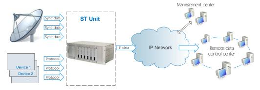
The unit is fully remotely configurable, by using FTP, WEB, SNMP features or proprietary NMS.
