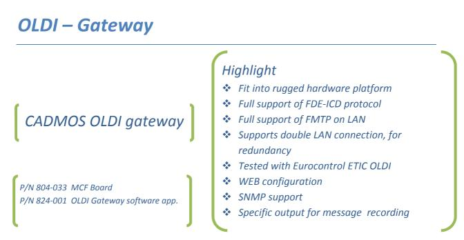
Now Cadmos ATC-router supports OLDI gateway function. This new application performs a bridge from legacy OLDI X25-FDE backbone to TCP/IP-FMTP infrastructure. CADMOS fills the gap of the FMTP specification in the current OLDI FDE-ICD applications
