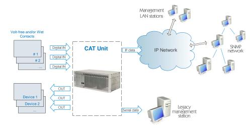
The unit is fully remotely configurable, by using FTP, WEB, SNMP or proprietary NMS.
